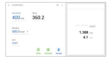
The spectrophotometer will calculate the factor so that this value can be used for future measurements.
