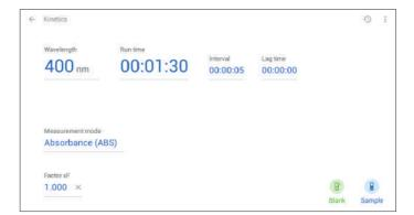
If a lag time has been set the instrument will count down the lag time before the kinetics run starts. If no lag time has been set the kinetics run starts straight away and a live kinetics run is shown on the screen.
