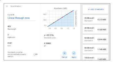
Specific points can be selected on the graph by touching the graph, a sliding cursor will appear. It is possible to move the cursor by dragging left or right.
