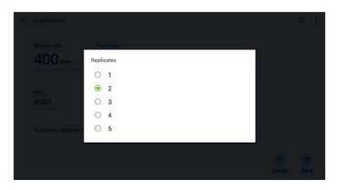
If 2 or more replicates are selected, Automatic replicates will read the same sample for the selected number of replicates. If individual sample replicates are being used, do not select the automatic replicates option.
