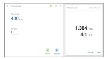
Once the measurement is complete the result will be shown. At this point you can either SAVE or UPLOAD.
