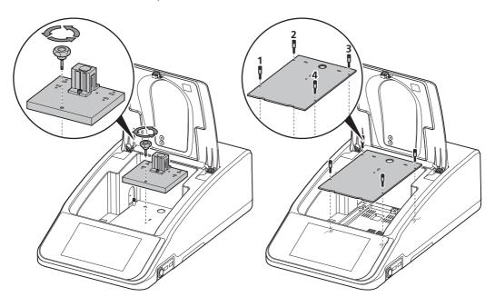
This will expose the bottom of the sample chamber and the power supply connection needed to operate the active accessories.
